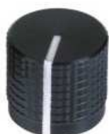
46154 Aluminum shell knob with ABS plastic insert, square knurl and indicator line on top and side Material: ABS Diameter: 10.16 mm Height: 10.2 mm Shaft hole: "D" type, \varnothing 6 x 4.34 mm
