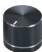
46107 Aluminum shell knob with ABS plastic insert and indicator line on top, microbrite chamfer and silver ring Diameter: 20 mm Height: 17.2 mm Shaft hole: \phi 6 mm, 18 Teeth
