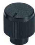
46095 Rotary knob with recess indicator line on top, straight knurl in outside, light texture on top Material: ABS Diameter: 15 mm Height: 12 mm Shaft hole: \phi 6 mm, 18 Teeth
