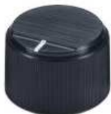
46110 Plastic knob with hair line polish on top with knurling and paint filled indicator line on top Material: ABS Diameter: 24.8 mm Height: 18.5 mm Shaft hole: \phi 6 mm, 18 Teeth
