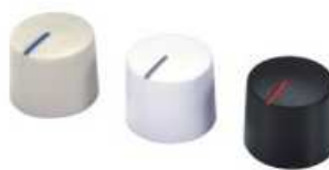
46103 Plastic knob with paint filled indicator line on top, EDM texture finish Material: ABS Diameter: 19.8 mm Height: 16.9 mm Shaft hole: \phi 6 mm, 18 Teeth
