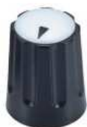
46116 Plastic knob with multi-color plastic cap, matte texture finish Material: ABS Diameter: 10.4 mm Height: 14.4 mm Shaft hole: \varnothing 6 mm, 18 Teeth
