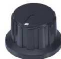
46148 Fluted plastic knob light texture finish indicator dot on top Material: ABS Diameter: 24 mm Height: 15.9 mm Shaft hole: \varnothing 6 mm, 18 Teeth
