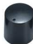
46144 Rotary knob with indicator dot on top, light texture finish Material: ABS Diameter: 12.6 mm Height: 13.5 mm Shaft hole: \varnothing 6mm, 18Teeth
