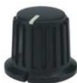
46152 Fluted plastic knob light texture finish indicator dot on top Material: ABS Diameter: 17.8 mm Height: 15.9 mm Shaft hole: \varnothing 6 mm, 18 Teeth
