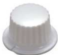
46124 Phenolic knob with ribs on O.D, glossy finish with one set screw Material: UREA, PHENOLIC Diameter: 23 mm Height: 14.6 mm
