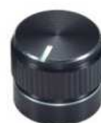
46108 Aluminum shell knob with ABS plastic insert and indicator line on top, microbrite chamfer and silver ring Diameter: 13.3 mm Height: 12.2 mm Shaft hole: \phi 6 mm, 18 Teeth
