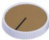
46146 Rotary knob with straight knurl on outside, Al. inlay on top Material: ABS Diameter: 31.7 mm Height: 6.4 mm Shaft hole: 6 x 4.5 mm with spring insert
