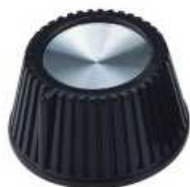
46138 Rotary knob with straight knurl on outside, pointer on side, Alum. Inlay on top Diameter: 25.1 mm Height: 15.5 mm Shaft hole: 6 x 4.5 mm with spring insert
