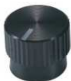
46105 Aluminum shell knob with ABS plastic insert straight knurl and indicator line on top Material: ABS Diameter: 11 mm Height: 10 mm Shaft hole: \phi 6 mm, 18 Teeth
