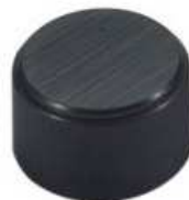
46111 Plastic knob with knurl and hair line polish on top Material: ABS Diameter: 30 mm Height: 20.5 mm Shaft hole: \phi 6 mm, 18 Teeth
