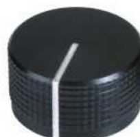
46155 Aluminum shell knob with ABS plastic insert, square knurl and indicator line on top and side Material: ABS Diameter: 16.5 mm Height: 10.2 mm Shaft hole: "D" type, \varnothing 6 x 4.34 mm
