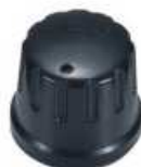
46143 Fluted plastic knob with indicator dot on top, gloss finish Material: ABS Diameter: 12.7 mm Height: 11.5 mm Shaft hole: 6 mm, 18 Teeth
