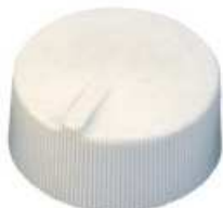
46139 Rotary knob with raised indicator line on top, straight knurls on outside, light texture on the top of knob Material: ABS Diameter: 26.7 mm Height: 14.2 mm Shaft hole: 6.4 x 5.6 mm with spring insert
