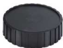
46092 Control knob with D type shaft and spring clip Material: ABS Diameter: 44 mm Height: 13 mm
