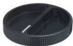
46096 Control knob with D type shaft and compression ring on O.D. Material: ABS Diameter: 37 mm Height: 15 mm
