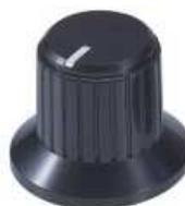
46147 Fluted plastic knob light texture finish indicator dot on top Material: ABS Diameter: 20 mm Height: 18 mm Shaft hole: \varnothing 6 mm, 18 Teeth
