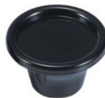
K112 Small knob w/name plate (glossy finish) 38x22.5 mm, hub dia. 10 mm, 10-32 UNF brass female insert Phenolic material
